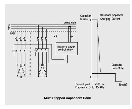
Such large-current can flow through contactor since initial in-rush current is taken from both mains-supply & capacitor already connected. As in-rush current of such high magnitude is undesirable & likely to weld main contacts of Standard Duty Contactors.
